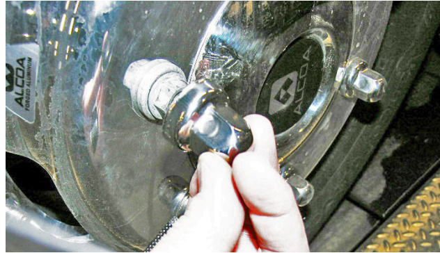
Remove the push on nut covers.
