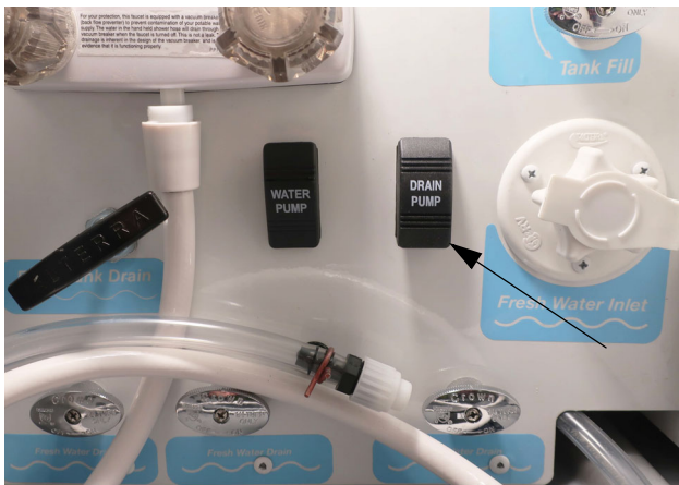
Waste Pump Switch (Located in water service center) -Typical View
