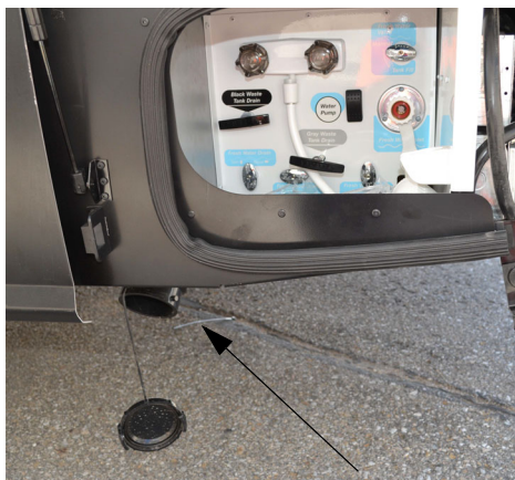
Sewage Drain Outlet (Located on the underside of water service center) -Typical View
